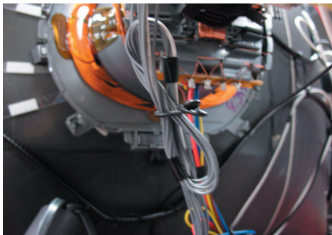
Dress RGB harness (A/CN301~ C/CN705) using a 9mm purple lock (3-703-982-02).
