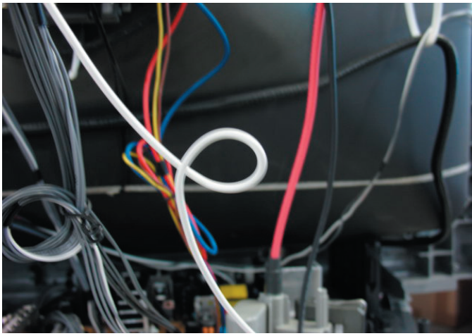
Dress G2 wire twist once as picture shown, do not over stress wire.
